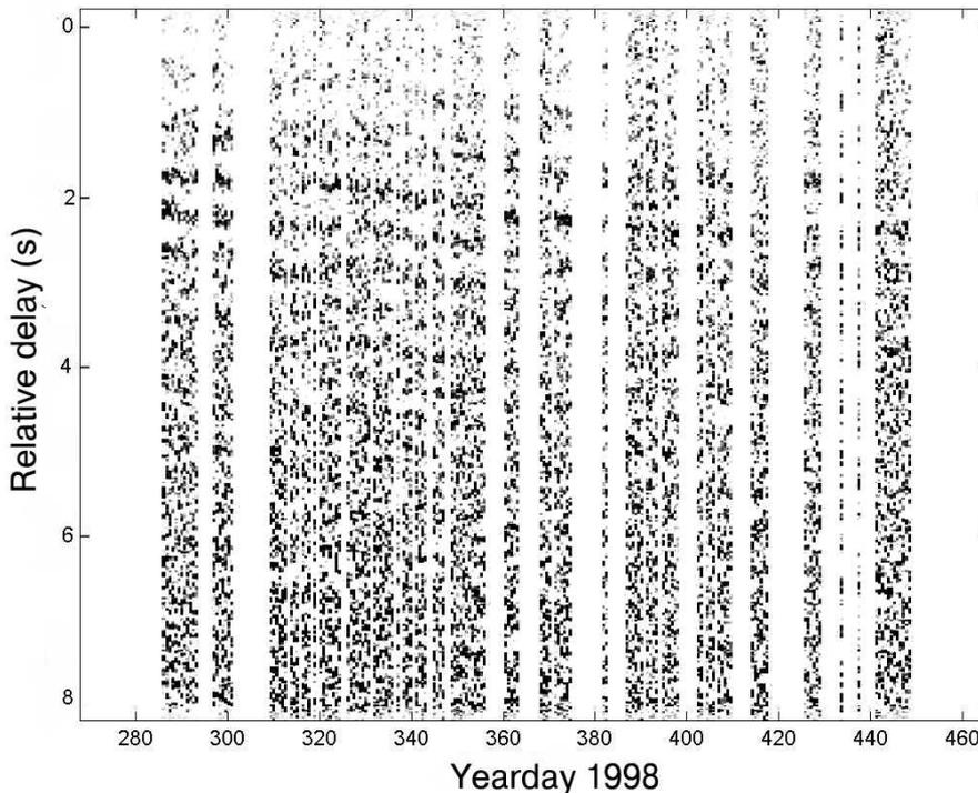
Figure 3. The signal level (displayed by blackening) after the processing as function of the time delay (vertical axis) and the day of 1998 (horizontal axis) Days with numbers exceeding 365 corresponds to year 1999.
