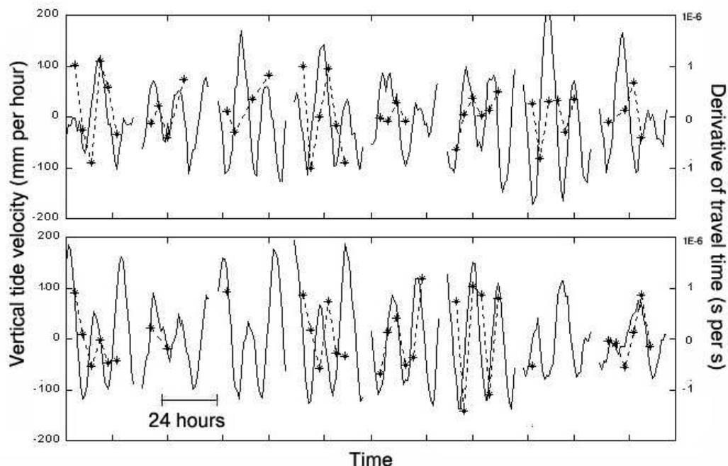
Figure 4. The rates of sea level changes near Hawaii (solid line and the left vertical scale) and the acoustic signal travel time (dotted line with crosses and the right vertical scale) for several days of 1998. The bottom plot is the continuation of the upper plot.
