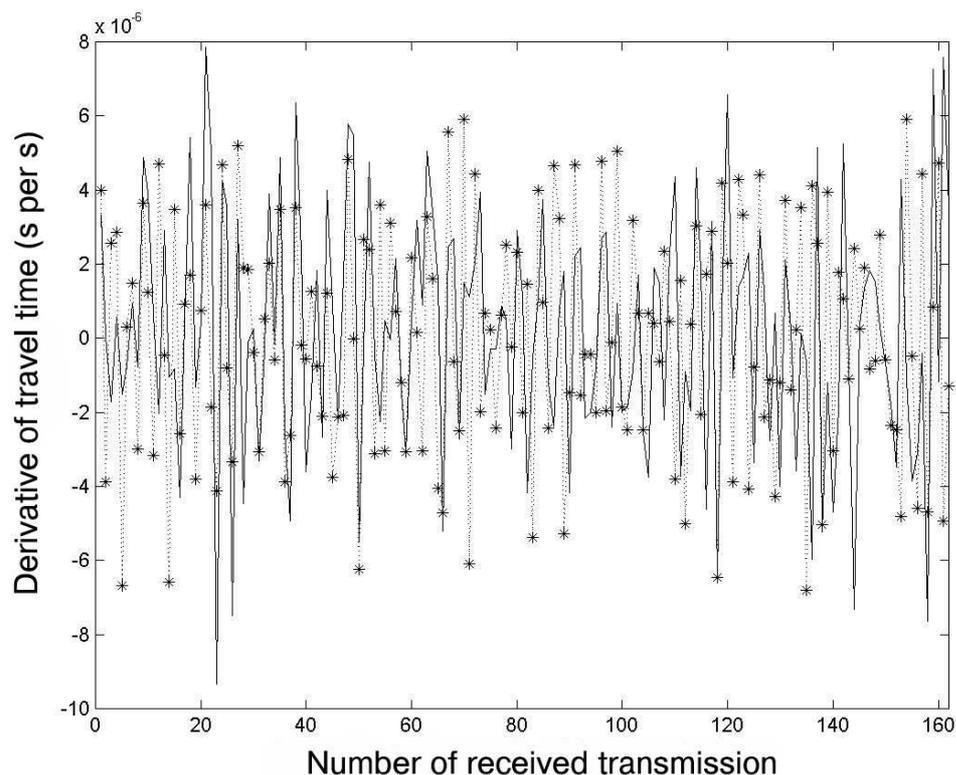
Figure 5. The rate of the travel time variations obtained from the observational data (dotted line and crosses) and from numerical calculations (solid line).
